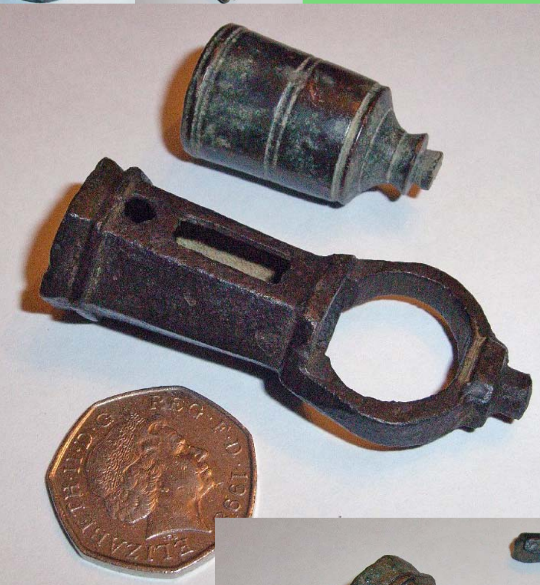
Figure 5 —Three possible casting failures, where smooth, rounded edges suggest the metal was not broken but failed to flow in the mould. Ring sockets are particularly prone to this, as their moulds were extremely narrow. The right-hand piece is a swan-neck attachment from a double-arm candlestick which lacks its socket attachment rings.
