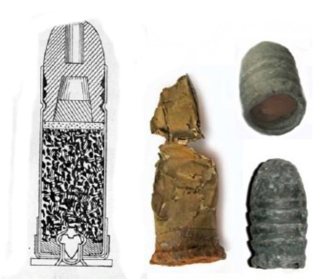
Figure 7 Graphic of a Boxer cartridge with the real thing alongside note the ceramic plug in the base of the bullet.
